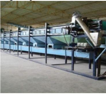
Manufacturer of Sago Dryers, dryer is used to remove the moisture content to the desired level. Used in the Sago dryers, Tea and other Spices industries.
